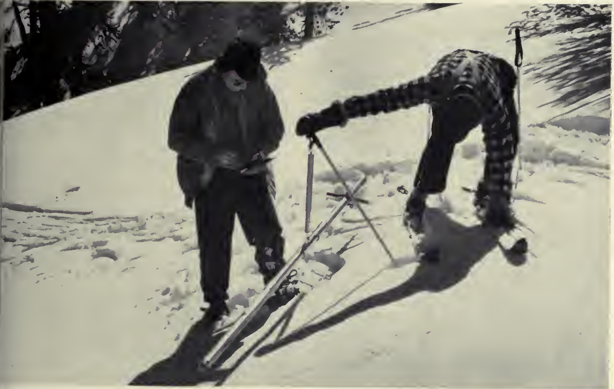
WHEN THE SNOW MELTS, how much water will run to the streams and fill the reservoirs? Snow surveyors find out by carefully weighing the hollow aluminum tube with its core of snow on specially calibrated scales. Photo by Robert Bronstead, courtesy of the Soil Conservation Service, United States Department of Agriculture.
